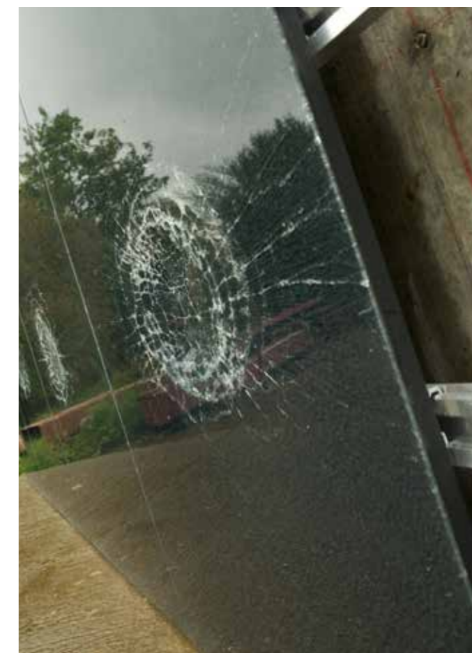
StoVentec Glass panels remain intact with little or no spalling after impact and explosion simulation
